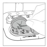
Lift the wiper membrane by using the recess on the edge. Remove the wiper and replace the brass wool with a new one. Make sure that the brass wool is on the far left and that there is space for the wiper on the right.
