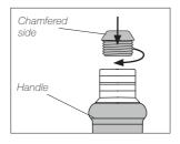
Position the chamfered side upwards and screw the new sealing plug into the handle bushing until it stops.
