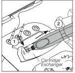
Place the tool with the cartridge over the cartridge exchanger slots and press down (1) until it clicks. To remove the cartridge pull the handle out (2).
