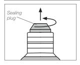
Remove the worn sealing plug by unscrewing it by hand.
