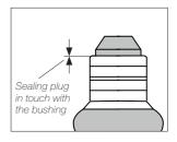
Make sure the sealing plug is placed correctly.
