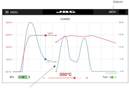
When the tool is not in use the graph stops recording
