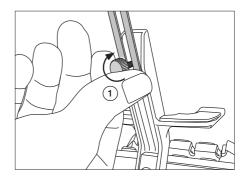
Insert the fixing knob (1) and tighten it just enough so that it stays in place but the display holder can be moved.
