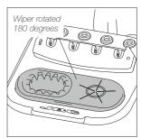
**Note:** The brass wool and the wiper positions can be reversed by rotating the antisplash membrane 180 degrees.
