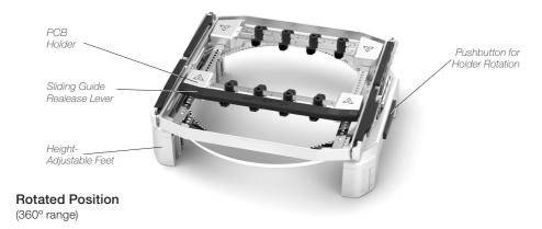
To rotate the PCB holder, press the lateral push button (1) to unlock its position. While the button is pressed, the holder can be rotated to the desired position (2). **Note:** In order to be able to rotate freely, the support needs to have a free space of at least 30 cm in diameter.
