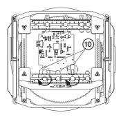
The clamp knobs can be loosened and tightened by hand and/or by means of the provided Allen key.
