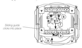
Now adjust the positions of the other requiered slot clamps to the PCB shape and tighten their clamp knobs (10) after the adjustment.
