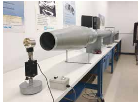
Wind Tunnel setup at Kanomax calibration lab
