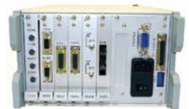
Model 1560 has 6 slots for modules
