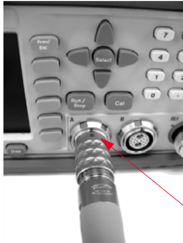
Figure 1-2 Connecting a sensor cable to a power meter
