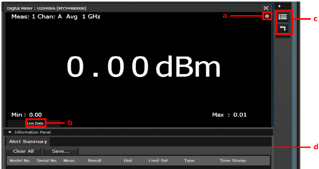
Figure 2-5 Average power meter measurement results
