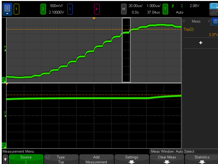
Figure 48 Isolating area for Top measurement
