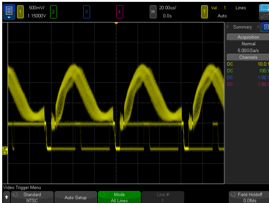
Figure 30 Triggering on All Lines
