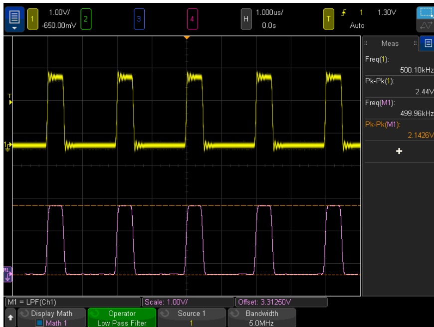
Figure 16 Example of Low Pass Filter
