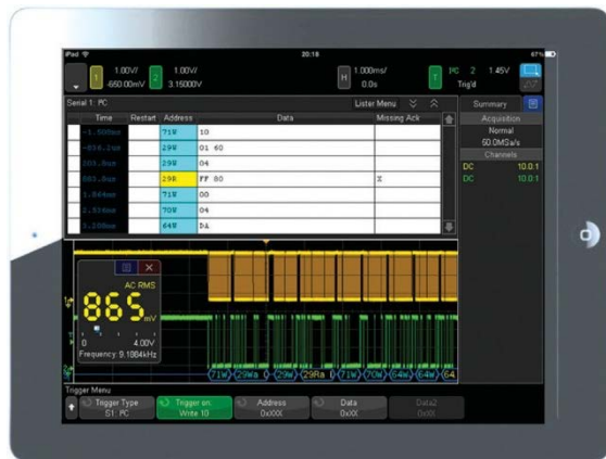
Figure 37. Tablet virtual front panel control.
