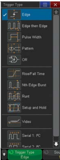
Figure 41. Wide array of advanced parametric trigger modes.
