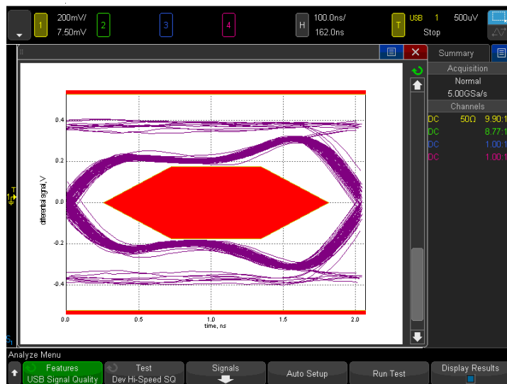
Figure 28. Perform automatic signal quality testing on USB 2.0 low-speed, full-speed, and hi-speed signals.
