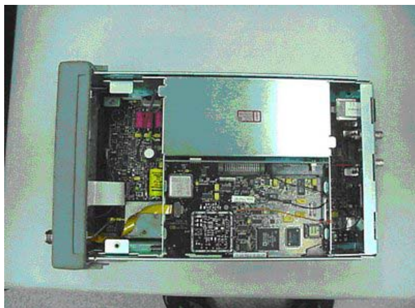
Figure A-4 Power meter with its cover removed
