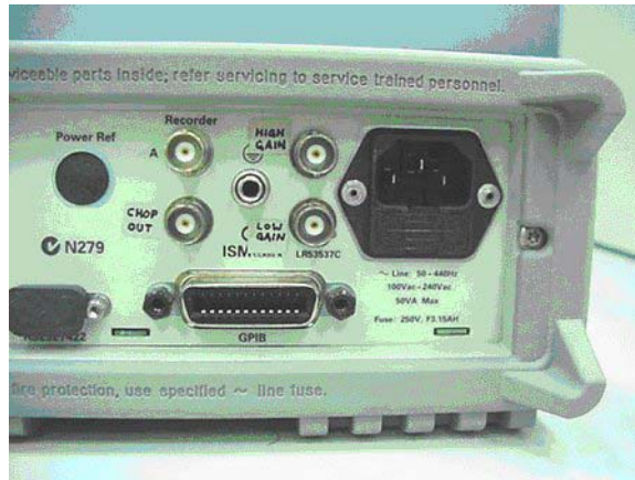
Figure A-11 Label the BNC connectors with a permanent marker and adhesive labels
