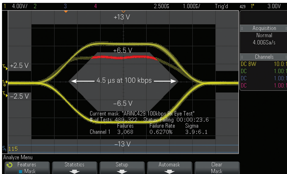
Figure 2. ARINC 429 eye-diagram mask test on 100 kbps data.
