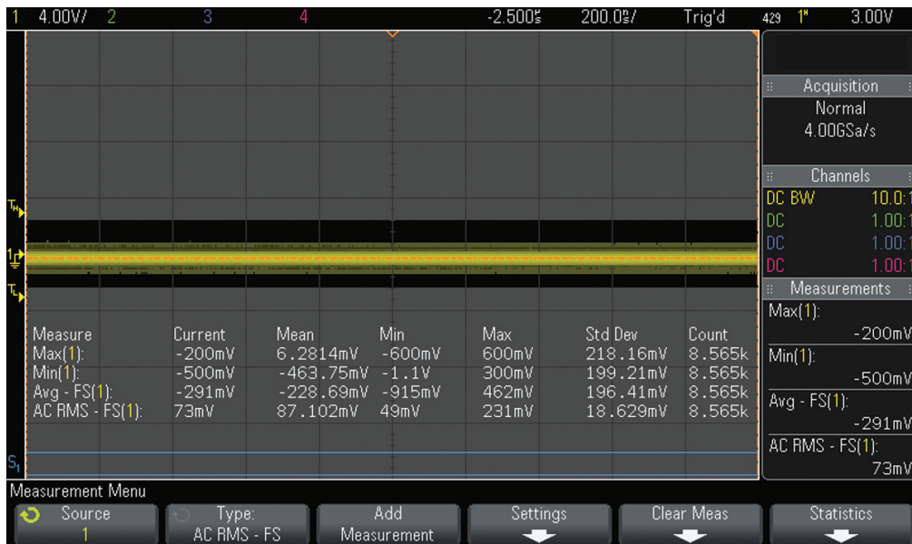
Figure 5. ARINC 429 “null” mask test with parametric measurements.
