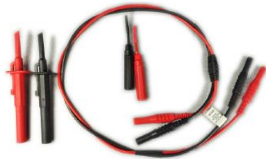
Figure 9. Extreme temperature probing kit.
