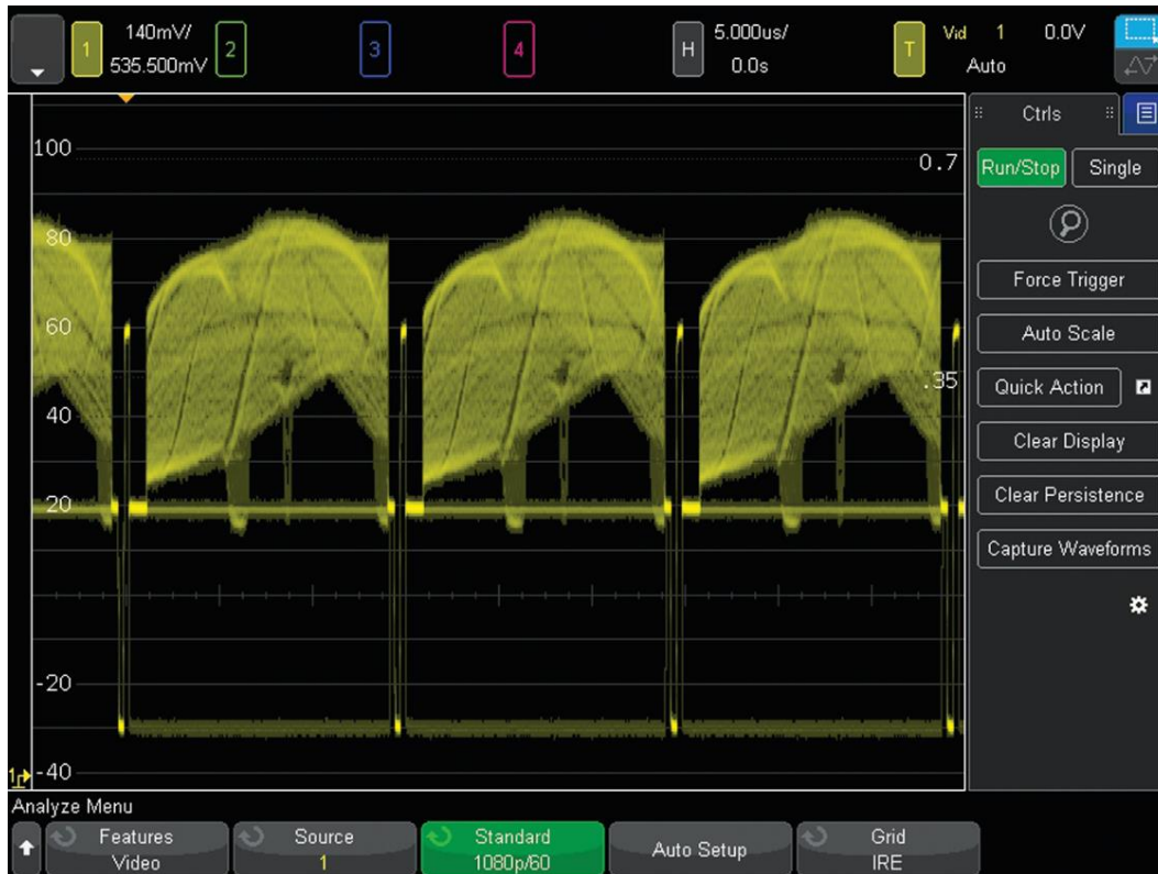
Figure 6. Triggering on 1080p HDTV.
