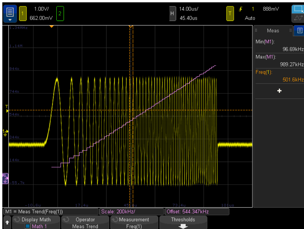
Figure 7. Measurement trend math function used to plot frequency versus time of a FM burst.
