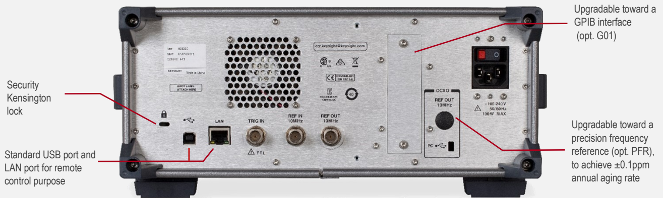
Figure 5. The rear panel of N932xC spectrum analyzer
