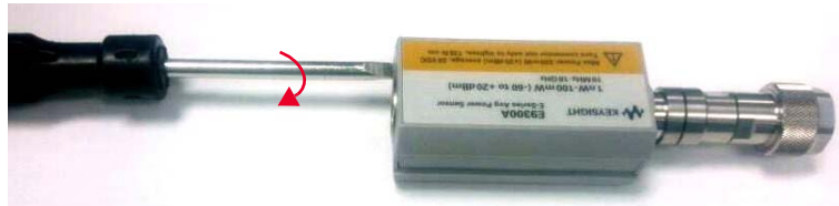
Figure 4-3 Removing power sensor shell
