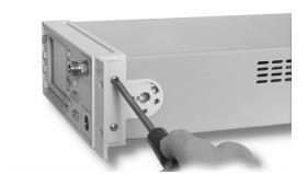
**5** Fit two front linking plates to each power meter.
