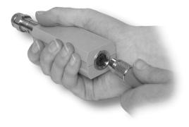
**2** Connect the other end of the E9288 Series cable to the CHANNEL A (or CHANNEL B) input connector.
