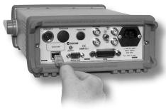
Recorder output (two outputs are fitted to dual channel meters) and Trigger Input and Output connections are made via BNC connectors.
