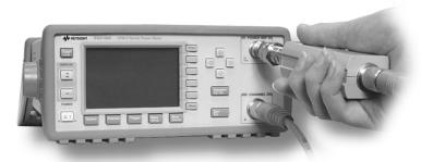
When the sensor is connected to the POWER REF, you can zero and calibrate the measurement path quickly by pressing Zero and Cal. On dual channel meters, press Zero + Cal A or Zero + Cal B.
