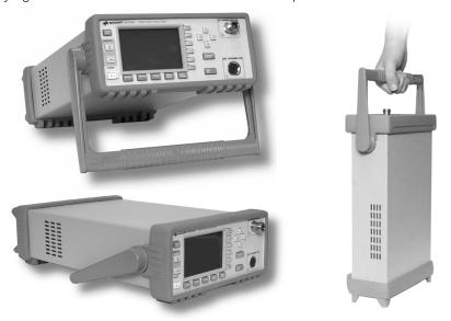
Pull the handle outwards, rotate it to the required position and release it into one of the three locks.
