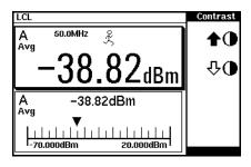
Figure shows display with an E-Series E9320 power sensor connected.
