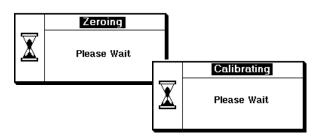
The **Zeroing** pop-up is displayed during the zeroing process, the **Calibrating** pop-up during calibration. The meter-sensor measurement path is calibrated when the **Calibrating** pop-up disappears.
