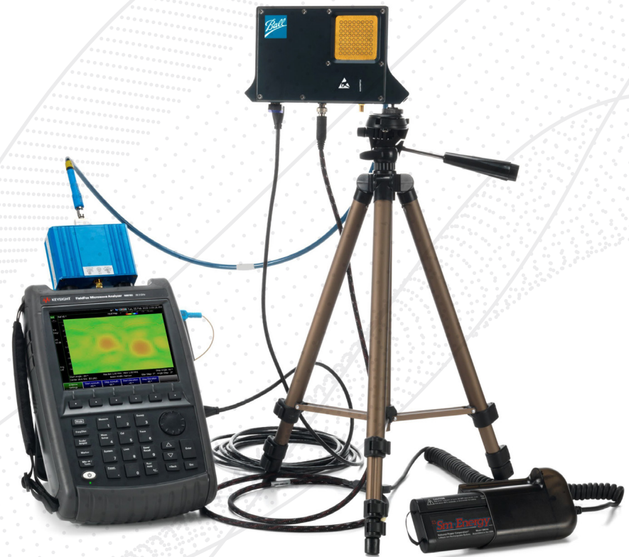
Figure 2. FieldFox and phased array antenna set up
