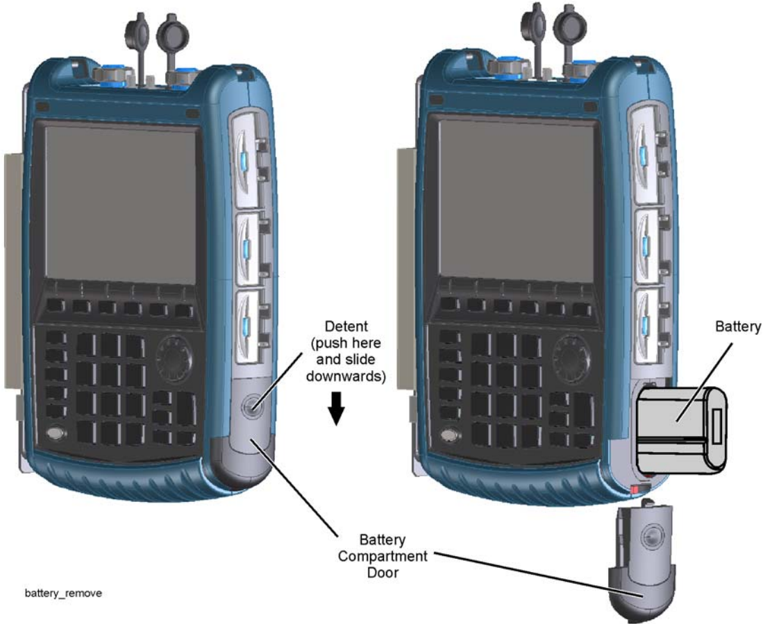
Figure 7-1 Replacing the Main Battery
