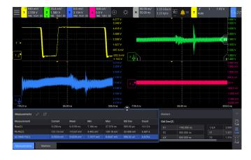
Utilize the full ADC and vertical resolution for every channel with split grids. Split FFT and math functions onto separate grids as well, letting you easily view and analyze your signals.
