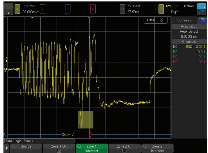
Figure 10: InfiniiScan Zone Trigger can be used to uniquely trigger on infrequent hi-speed USB signal problems.
