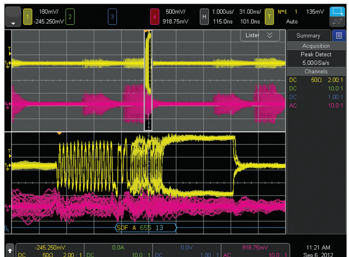
Figure 6: Poor PC board layout resulted in power supply switching noise coupling into one side of the hi-speed USB differential bus.
