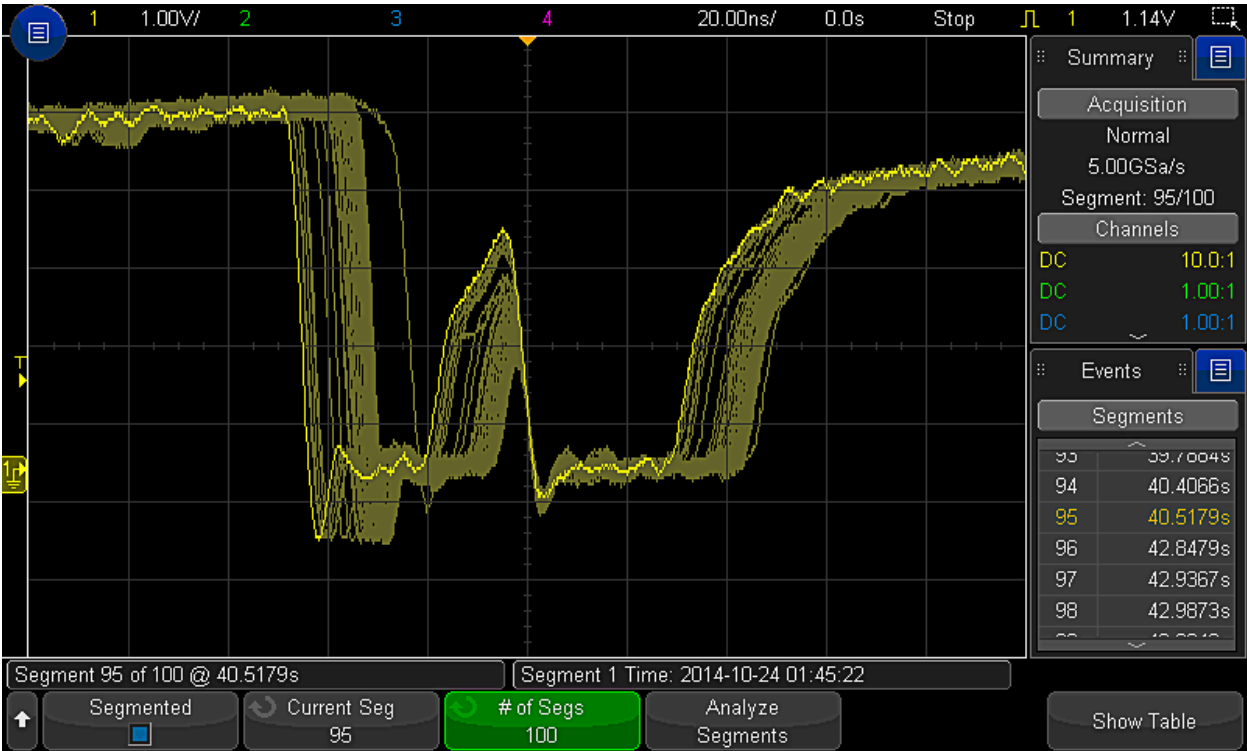
Figure 13a. Screen showing an overlay of all 100 segments for worst case waveform analysis.
