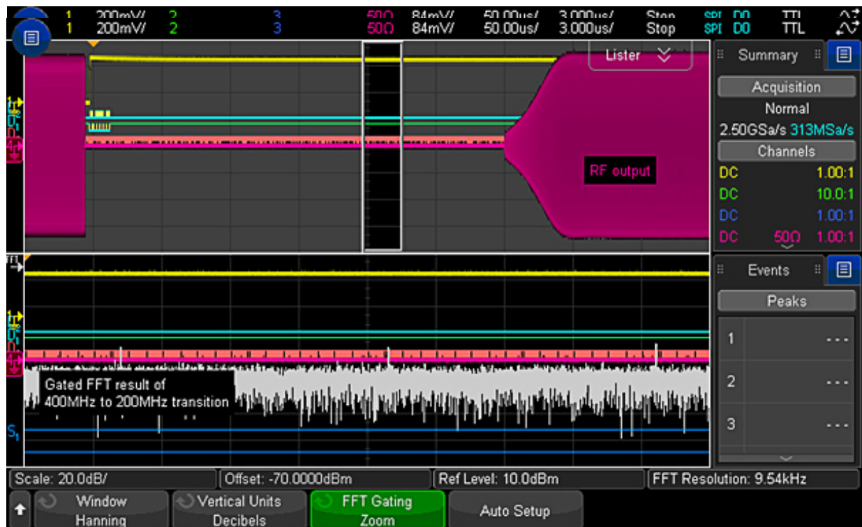
Figure 21a. Triggered on a SPI command, the RF signal is still at 400 MHz as indicated in the frequency peak search result lister.
