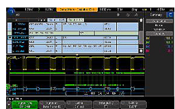
Figure 19. Multi-bus time aligned decode.
