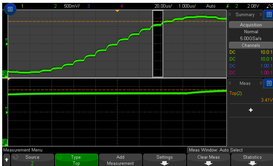
Figure 48 Isolating area for Top measurement
