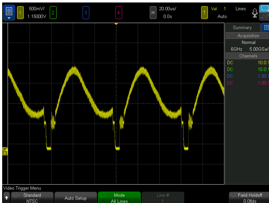
Figure 30 Triggering on All Lines
