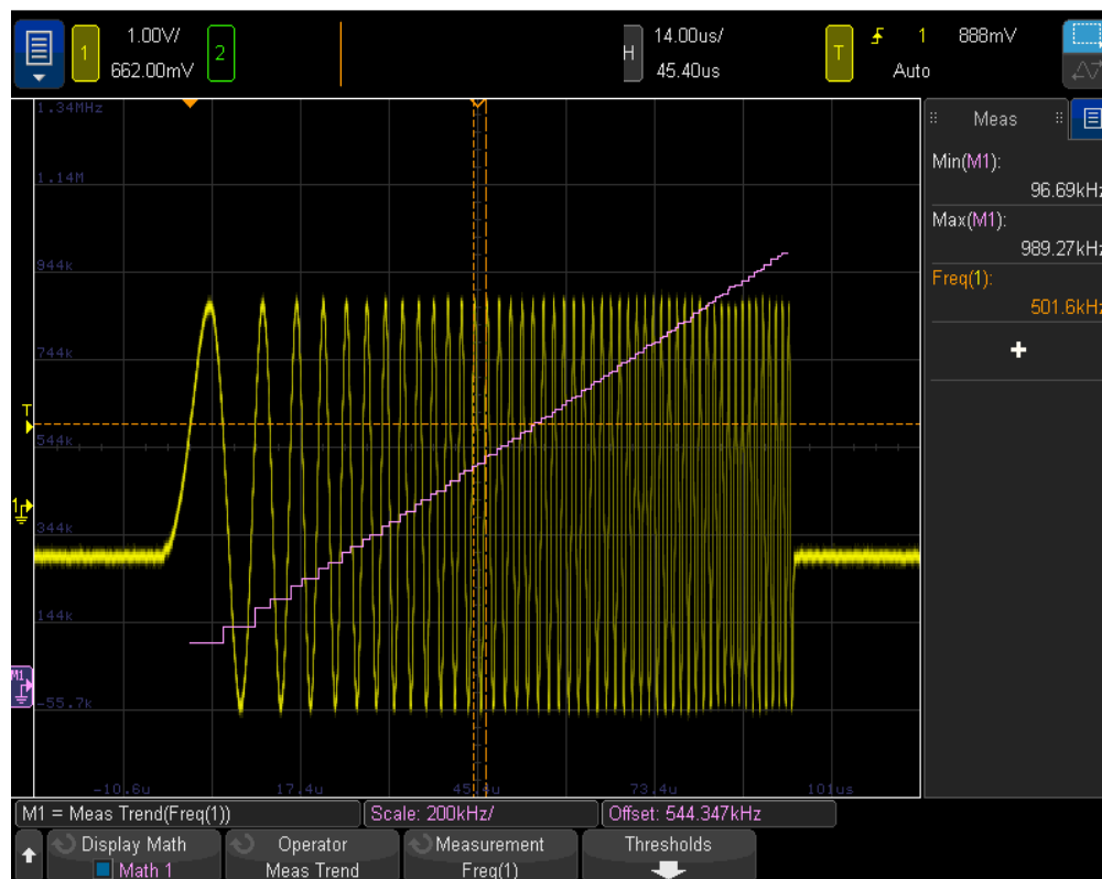
Figure 10. Measurement trend math function used to plot frequency versus time of a FM burst.
