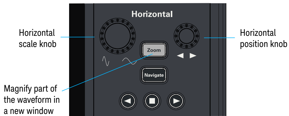
Figure 14 Front panel horizontal knobs and controls
