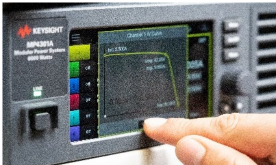
Figure 4. Intuitive touch display, setting SAS curve
