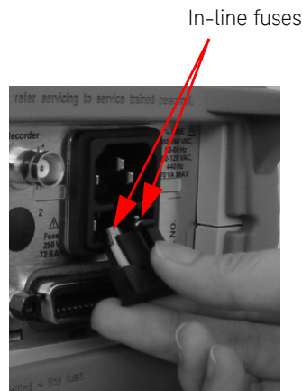
Figure 3-4 Checking the fuses
