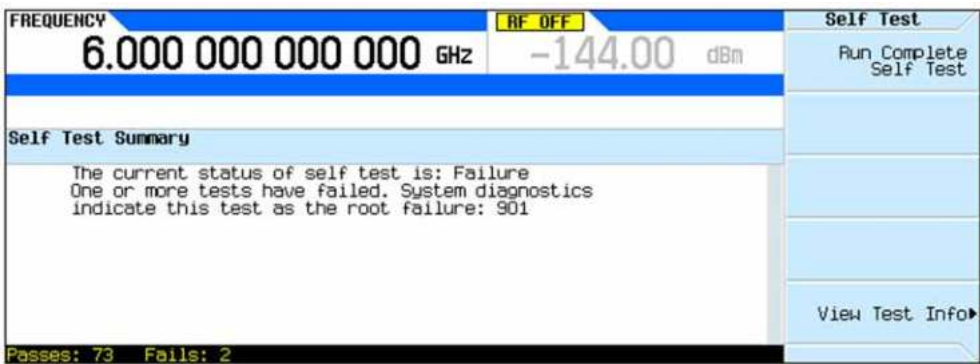
Figure 4-5 Self Test Failure Message
