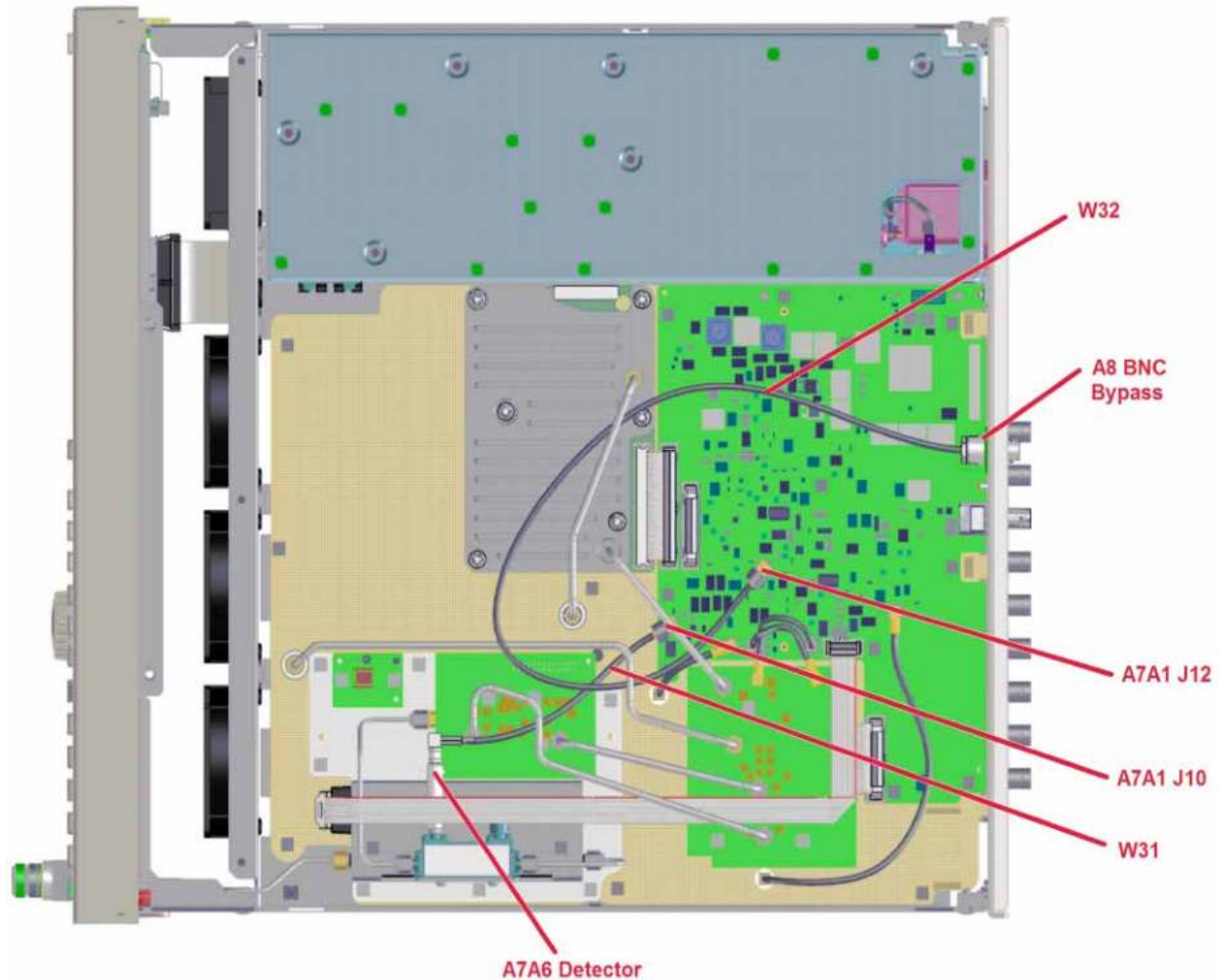
Figure 6-4 External ALC Leveling Loop
