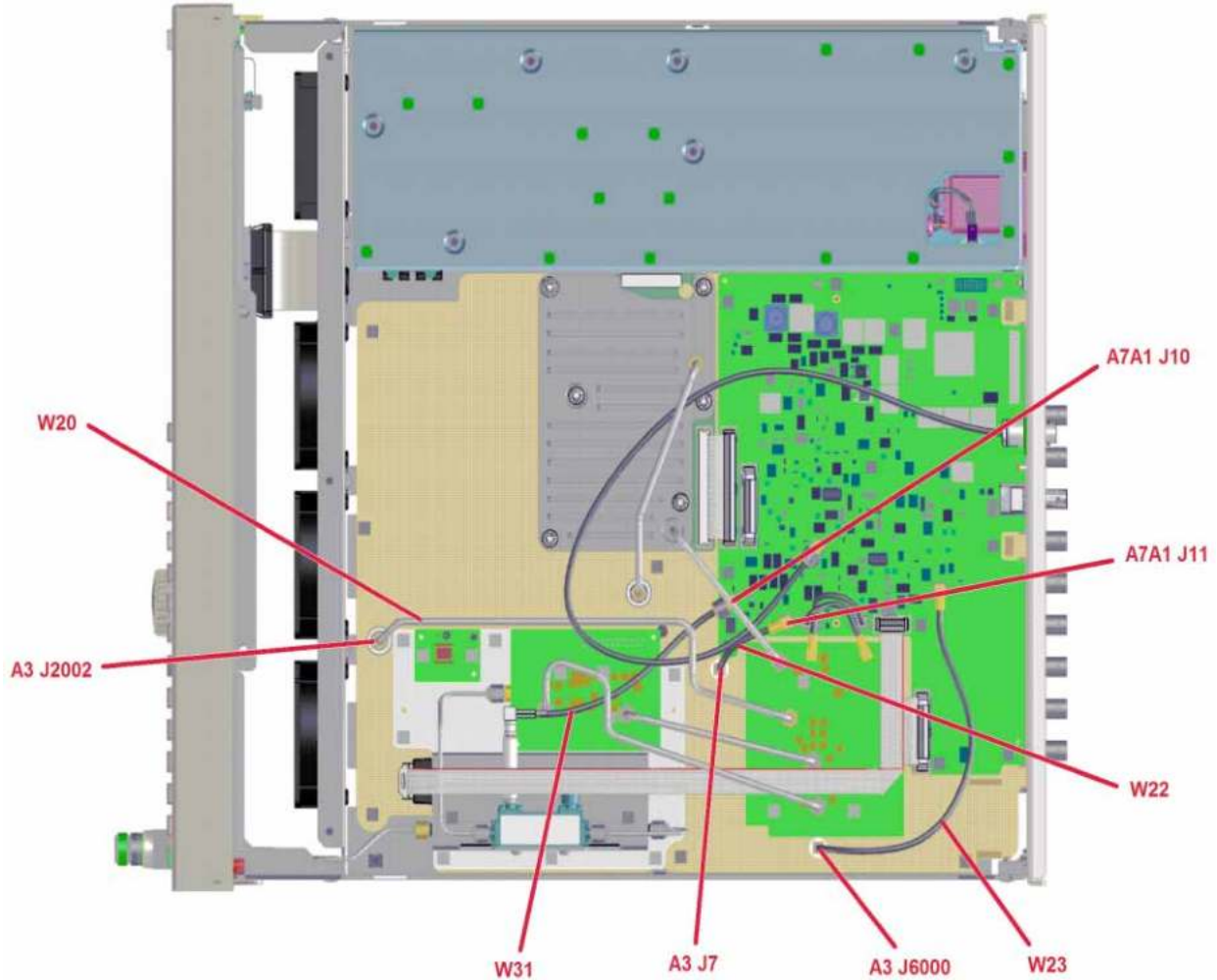
Figure 6-2 Less Than 3.2 GHz Internal ALC Leveling Loops
