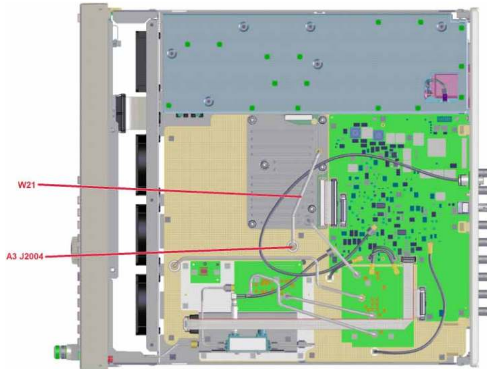
Figure 10-4 Synthesizer Multiplier / Divider Section Output - Microwave
