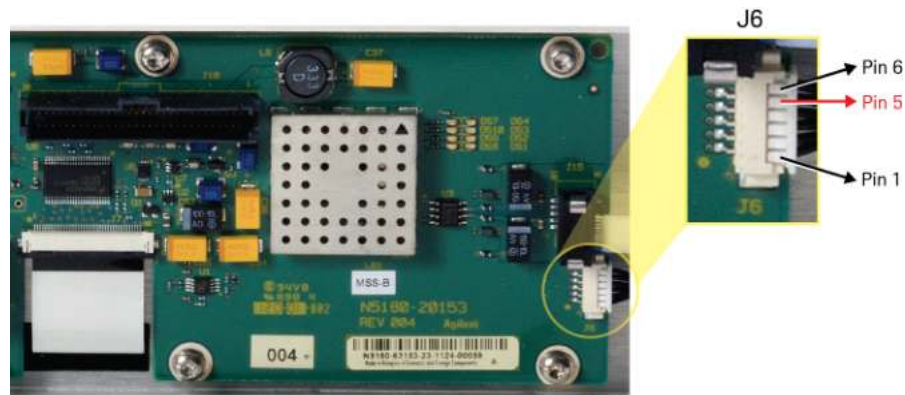
Figure 2-2 A6A1 Front Panel Interface J6 Pinout
