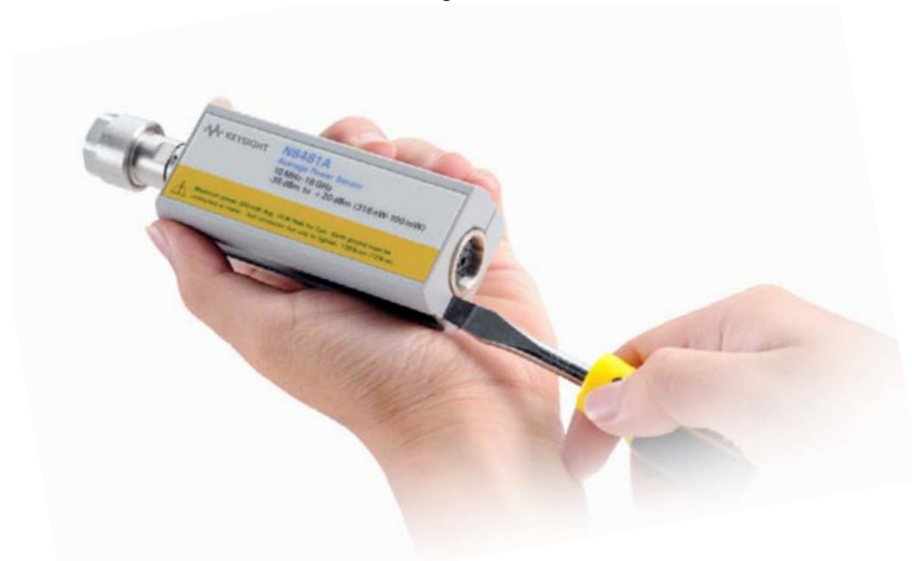
Figure 3-2 Removing the power sensor shell
