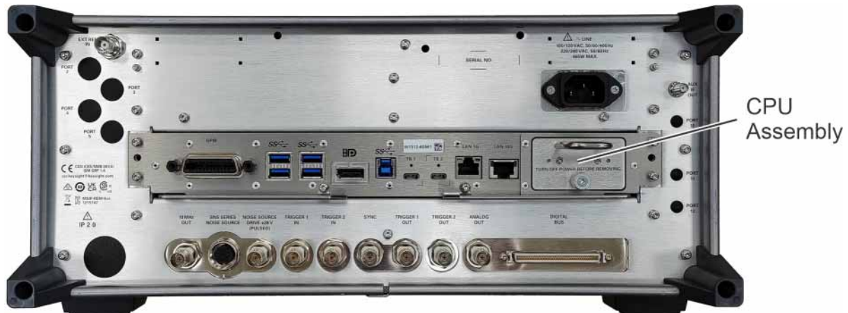
Figure 15-56 CPU Assembly - Rear Panel View
