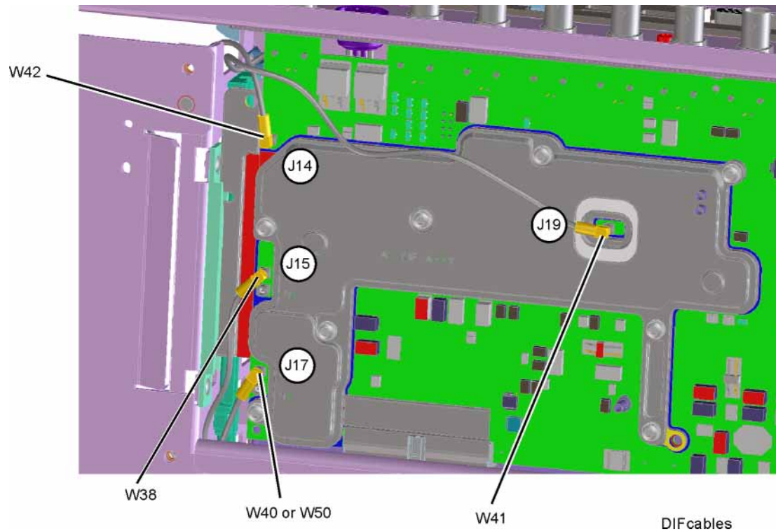
Figure 15-63 W38, W40, W41, W42 Removal - Option B40, MPB, or DP2
