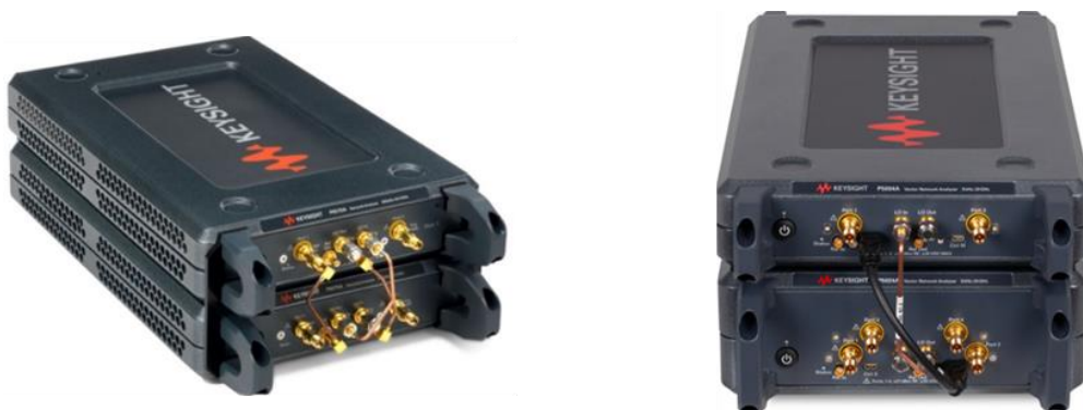
4-port configuration using two P937xA VNAs (left), 6-port configuration using 2-port P500xA and 4-port P502xA (right).
