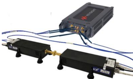
E-band VNA solution using P502xA and N5252AW frequency extenders.
