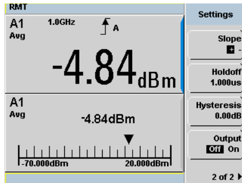
Figure 2-40 Trigger setting menu 2 of 2
