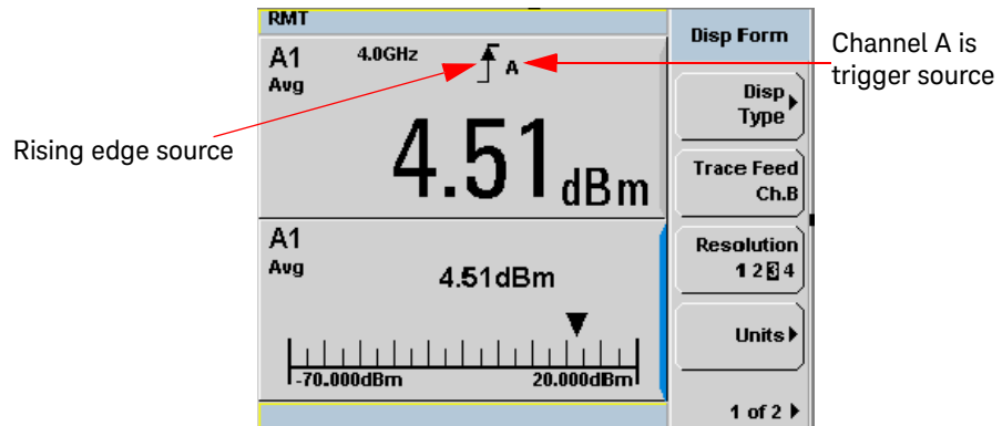
Figure 2-37 Trigger Setting Menu 1 of 2
