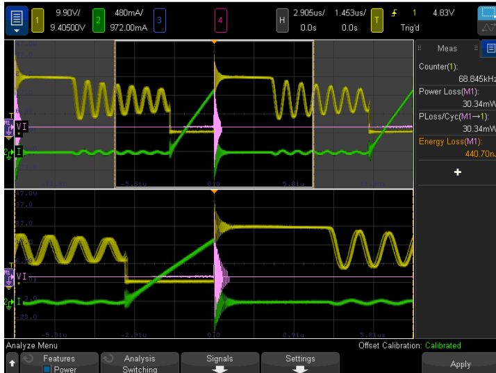
Figure 3. Power and energy loss measurements.
