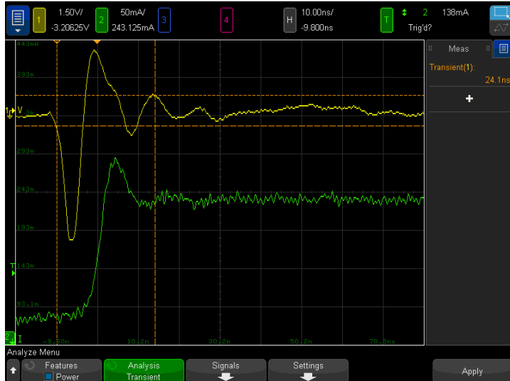
Figure 8. Transient response settling time measurement.
