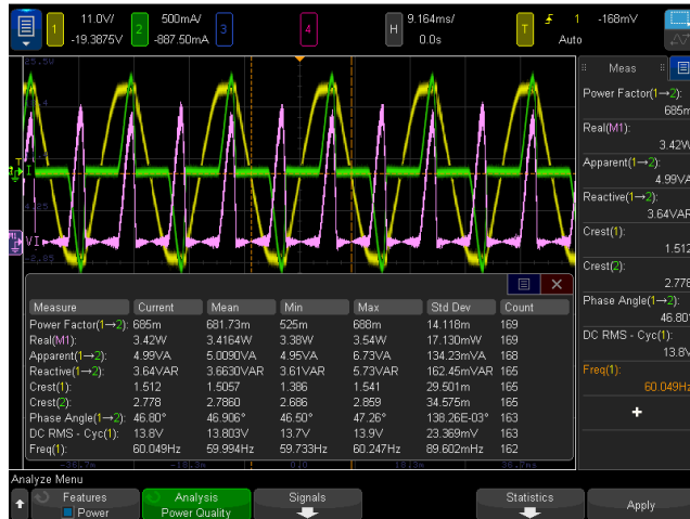
Figure 1. Input AC power quality measurements.
