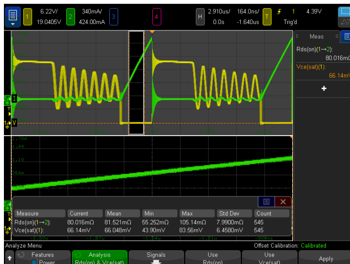
Figure 4. R_{DS(ON)} and V_{CE(SAT)} measurements.
