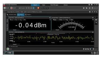
The U8480 Series is supported by the Keysight BenchVue software BV0007B Power Meter/Sensor Control and Analysis App. Control your USB power sensor to log data and visualize measurements in a wide array of display options.
