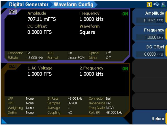
Figure 3-33 Digital Generator > Waveform Config menu page (square waveform)
