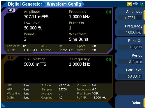
Figure 3-37 Digital Generator > Waveform Config menu page (sine burst)
