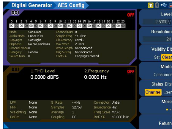
Figure 3-71 Digital Generator > AES Config menu page 1
