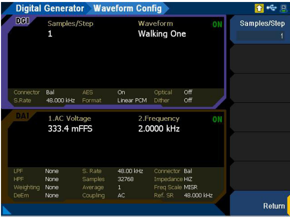
Figure 3-44 Digital Generator > Waveform Config menu page (walking one)
