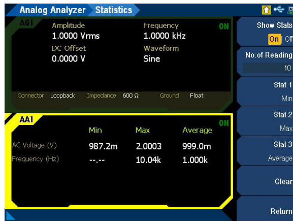
Figure 4-70 Analog Analyzer > Statistics menu page
