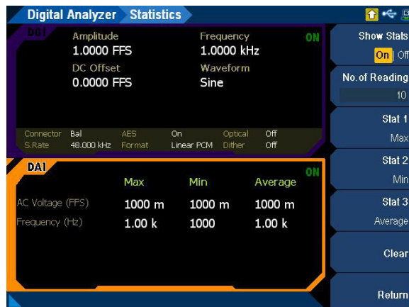
Figure 4-71 Digital Analyzer > Statistics menu page
