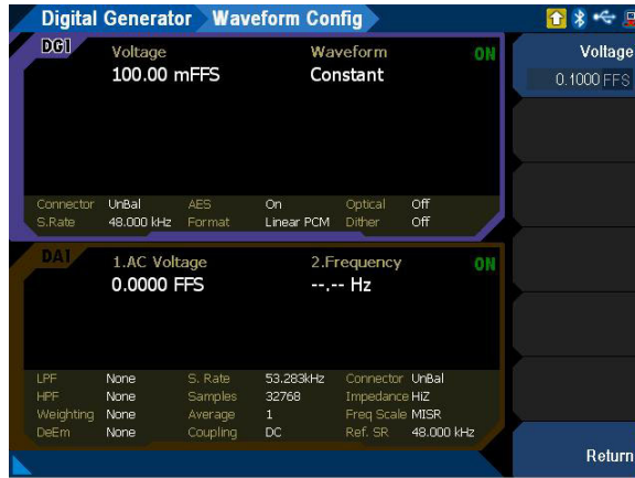
Figure 3-41 Digital Generator > Waveform Config menu page (constant)
