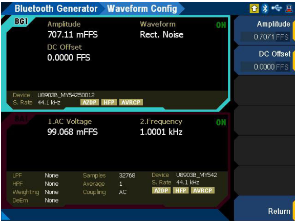
Figure 3-27 Bluetooth Generator > Waveform Config menu page (Rectangular noise)
