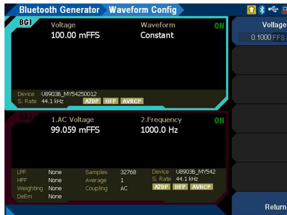
Figure 3-42 Bluetooth Generator > Waveform Config menu page (constant)
