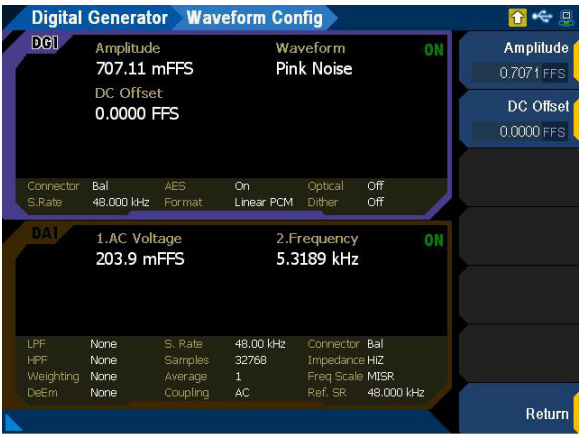
Figure 3-30 Digital Generator > Waveform Config menu page (Pink noise)
