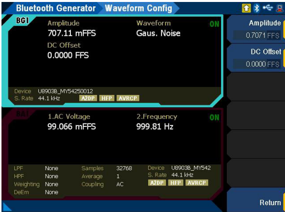
Figure 3-24 Bluetooth Generator > Waveform Config menu page (Gaussian noise)
