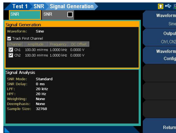
Figure 7-23 SNR > Signal Generation settings menu page
