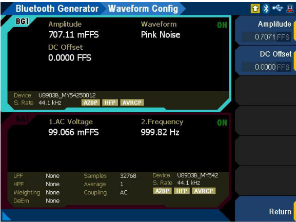
Figure 3-31 Bluetooth Generator > Waveform Config menu page (Pink noise)
