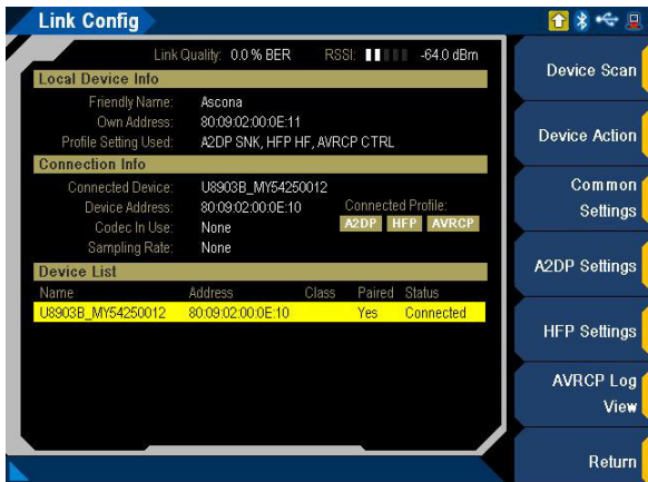
Figure 3-61 Bluetooth Generator > Link Config menu page
