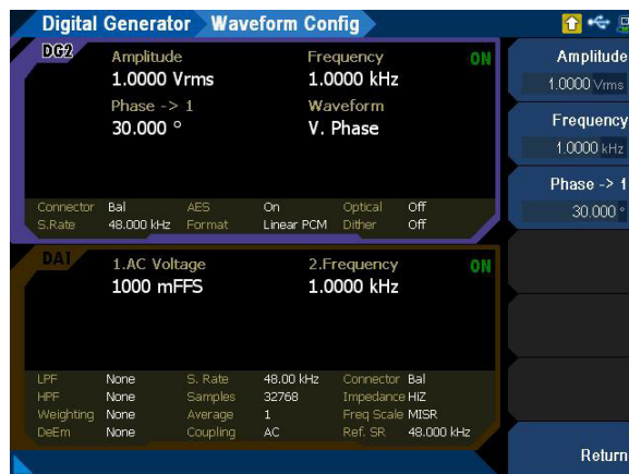
Figure 3-8 Digital Generator > Waveform Config menu page (variable phase waveform)
