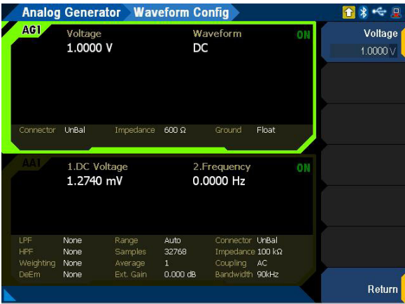
Figure 3-35 Analog Generator > Waveform Config menu page (DC signal)
