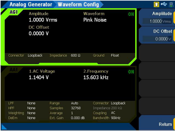
Figure 3-29 Analog Generator > Waveform Config menu page (Pink noise)
