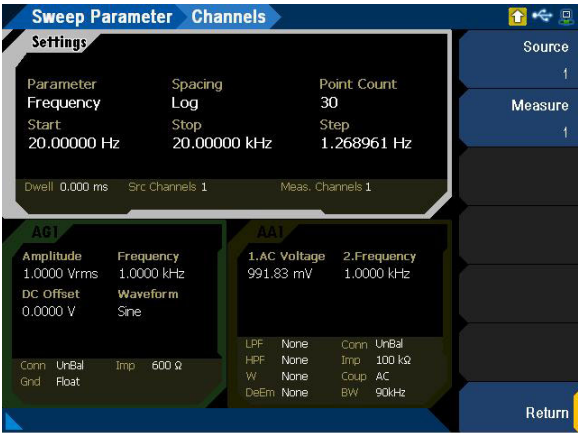
Figure 6-4 Sweep Parameter > Channels menu page
