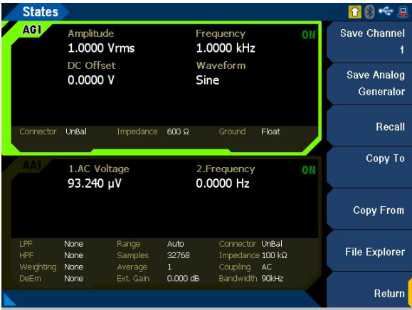
Figure 2-22 Utility menu page (generator and analyzer mode)
