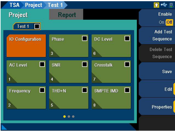
Figure 7-5 TSA > Project > Test menu page
