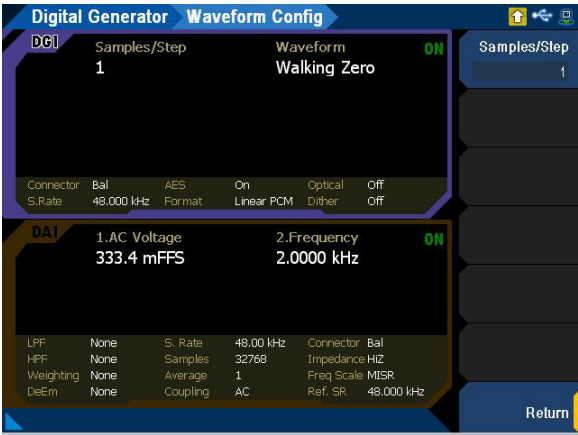
Figure 3-43 Digital Generator > Waveform Config menu page (walking zero)
