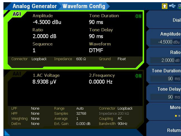
Figure 3-54 Analog Generator > Waveform Config menu page 1 (DTMF)
