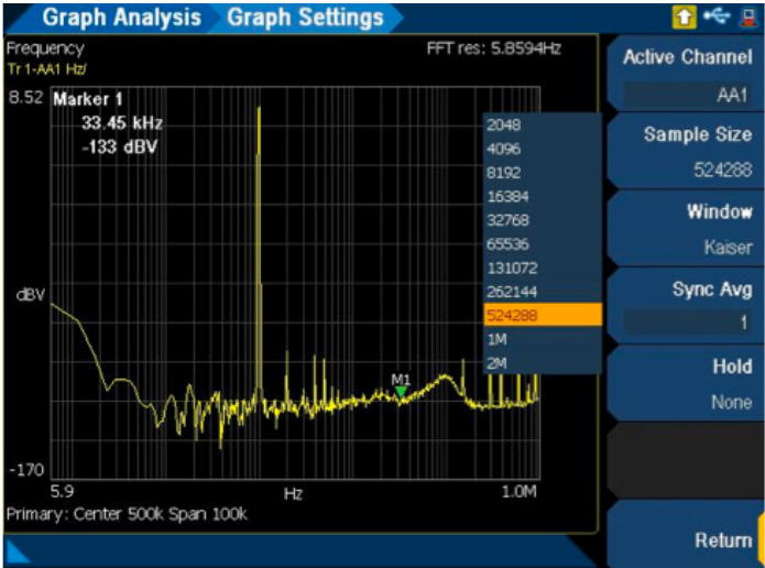
Figure 13. FFT with 524288 sample size
