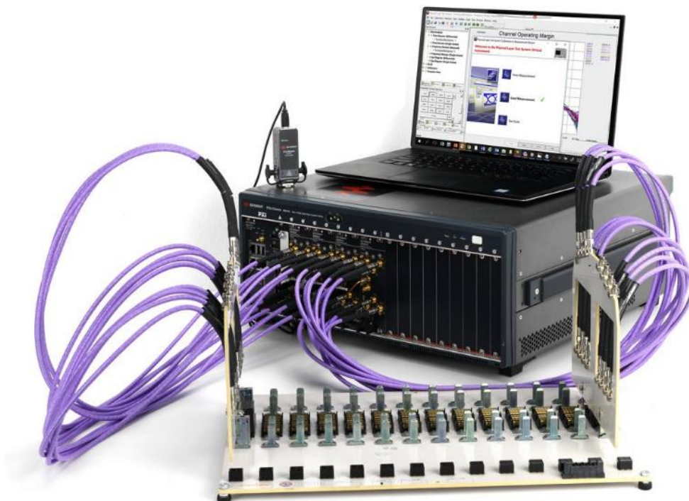
Figure 4. M980xA PXI VNA meets the most demanding multiport challenges with a true multiport architecture.
