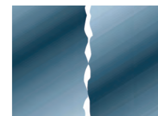
Typical interference fit has 30% metal-to-metal contact.
