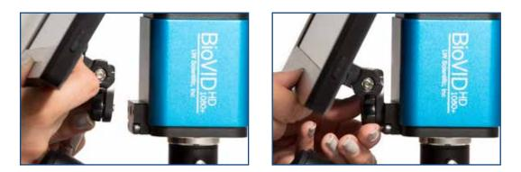
Remove the monitor from its packaging and mount the monitor to the camera's front mounting bracket using the included thumbscrew. Do not overtighten the thumbscrew but ensure you securely tighten it to prevent the monitor from falling off of the camera.
