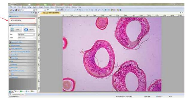
3 At this point, the screen should be showing a live image from the microscope. If not, look at the microscope head and check if there is a pull knob that directs light up to the trinocular head.
