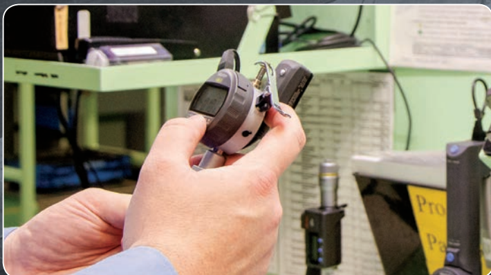
Inspection being performed at the point of manufacture. Sampling techniques based on capability reduce the time spent on inspection while still ensuring the quality of the product.
