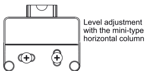
Fix with ST4 × 20mm self-tapping screw
