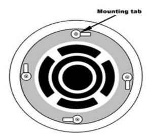
Be sure to position the four Mounting Tabs on your OWI speaker inward then insert the four (4) screws (supplied) from the front of the speaker into the screw opening.
