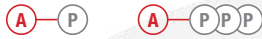
One OWI Amplified Speaker Can Power One Or Up To Three Passive Speakers
