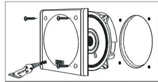
Both the M5CX and M4F weatherized speakers are held in place by (4) #8 stainless steel screws. Locate the speaker grill covers and put a small amount of silicone in screw holes. This will seal the screws. Using the Philips screw driver, install the (4) #8 screws carefully aligning speaker in wall. (It is not necessary to seal the speaker grill cover - only the screw holes.)
