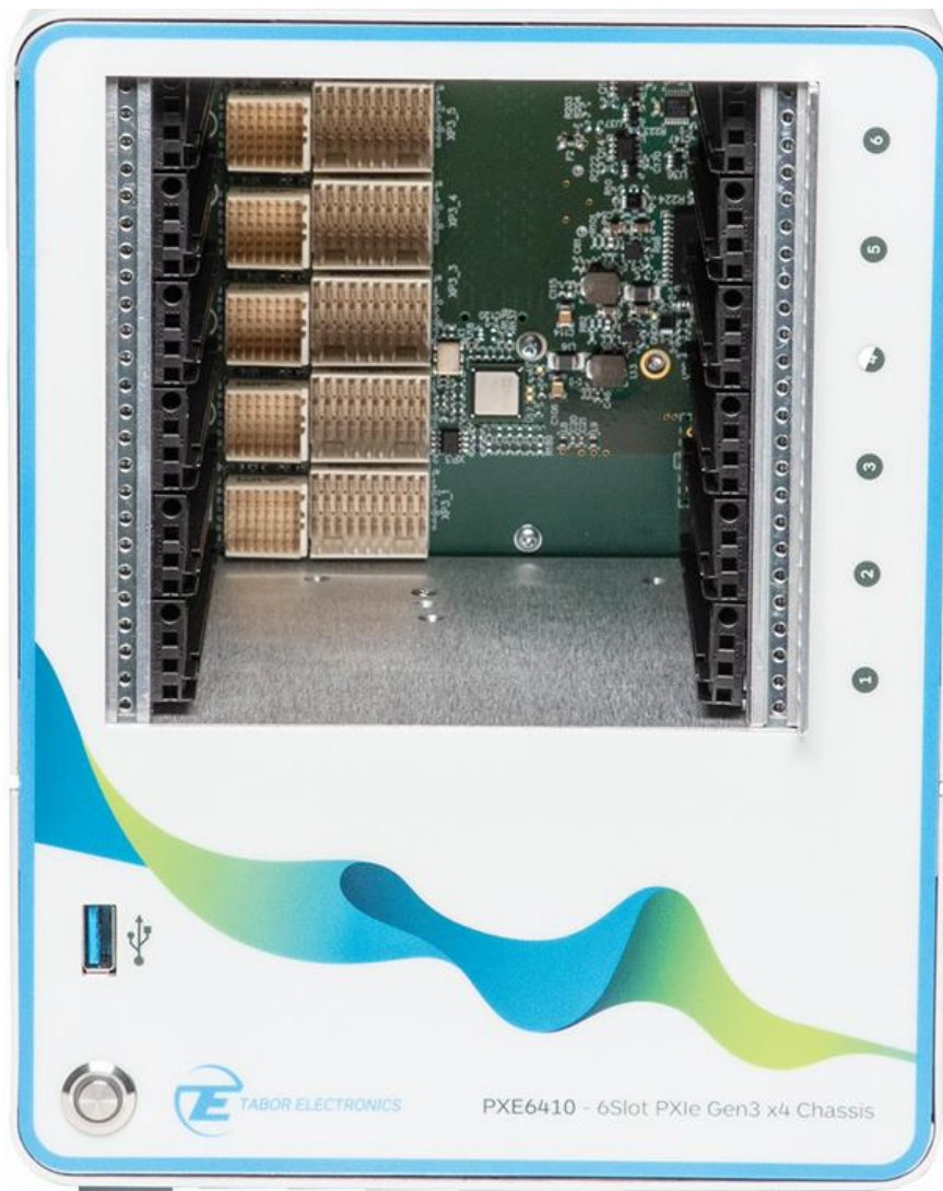
Figure 2.2 PXE6410 Front Panel
