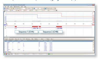
We can see two address-data-data sequences on the  $I^2C$  bus in the scope view, together with the decoded data in the lower window. Both sequences begin with the DAC's address, 0C. The first sequence (0C-01-24-1D) addresses the device's CHA output and causes it to change level. The second sequence (0C-02-24-1D) repeats this operation for the DAC's CHB output.
