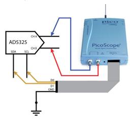
We captured some I<sup>2</sup>C packets using digital channel D0 for SCL (clock) and D1 for SDA (data). In the *Tools* menu we selected *Serial Decoding* and then set channel A to decode I<sup>2</sup>C data. We checked the *In View* and *In Window* boxes to view our data in both graphical and tabular formats, and clicked *OK*.
