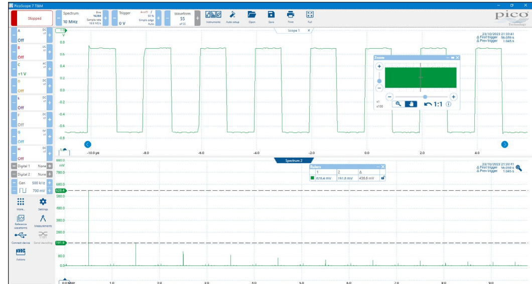
Harmonics of a square-wave signal
