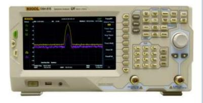
Figure 1: Rigol DSA815-TG Spectrum analyzer.
