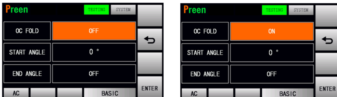
Figure 3.12 Enable the o OC-FOLD mode
