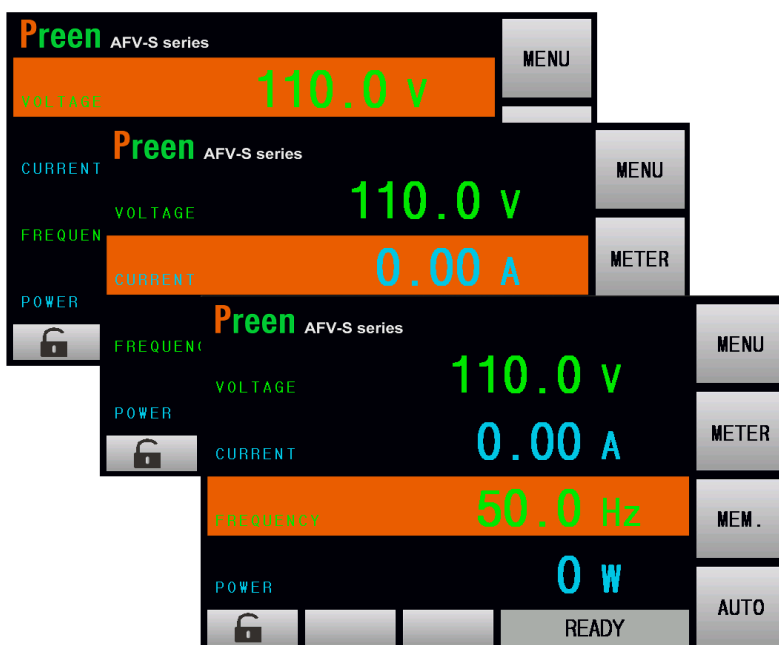
Figure 3.3 Move the cursor on the touch screen by turning the rotary knob
