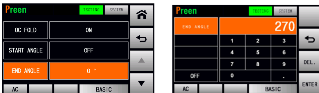
Figure 3.14 Set the end angle from 0° to 270°
