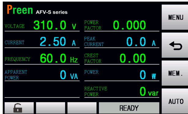
Figure 3.48 METER page when the output is on
