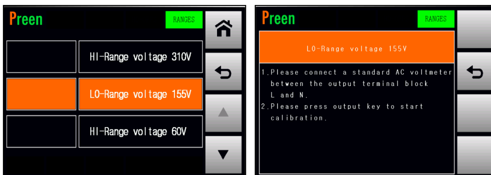
Figure 4.7 Enter the page which calibrates the LO-Range voltage 155V
