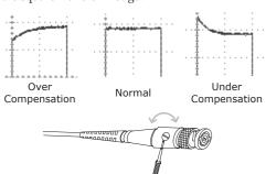
11. Setting up the oscilloscope is complete. You may start to use the oscilloscope.
