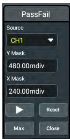
Figure 16.2 Minimized Pass/Fail Test Window
