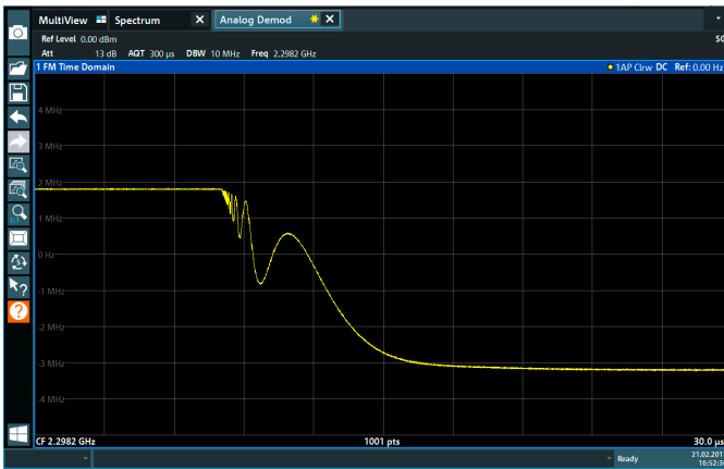
Frequency settling behavior of an oscillator
