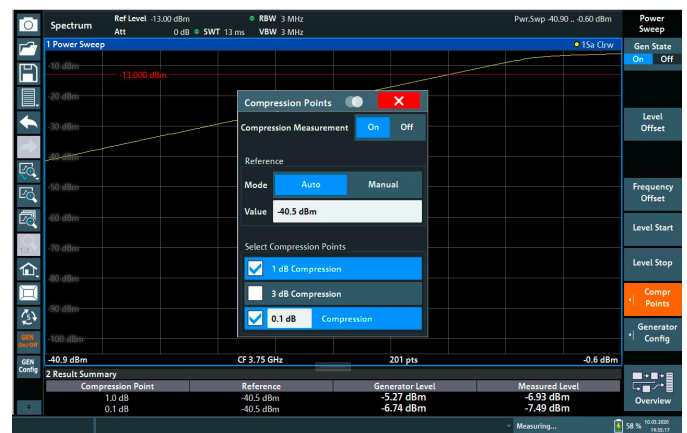
Measurement of 1 dB and 0.1 dB compression points
