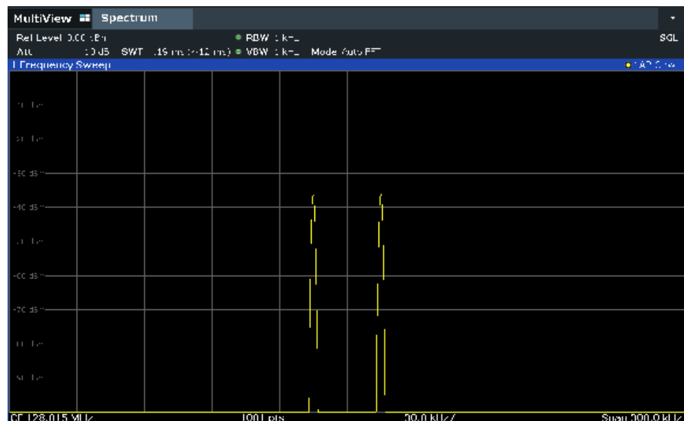
Figure 6-8: Measurement of two equally-leveled RF sinusoidal signals with a resolution bandwidth (1 kHz) which is significantly smaller than their frequency spacing
