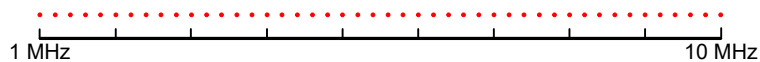
Figure 6-43: Linear x-axis scaling: the distance between the sweep points is equal, e.g. 200 kHz
